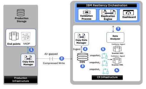
This CIR capability enables recovery against cyberattacks that corrupt the data. It allows replication of the data from servers and storage using copy data management solutions, with an airgapped mechanism, into an immutable storage located in the Cyber site of the customer and maintains multiple read-only PIT copies.
