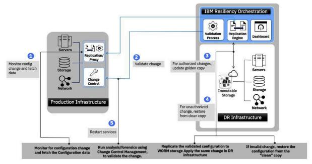
This CIR capability enables recovery against cyber It replicates the configuration data of these devices attacks that corrupt the configuration and alter the and servers with an air-gapped mechanism, into behaviour of data center platforms including network devices, storage devices and virtual or physical servers.
